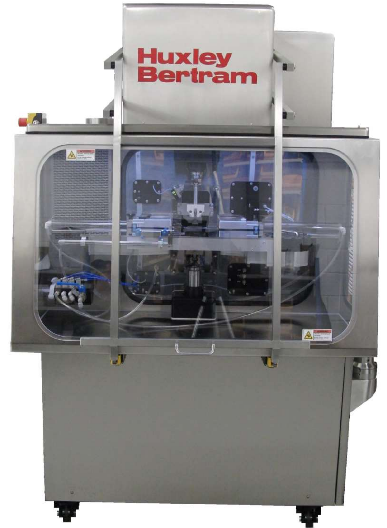
The Huxley Bertram hydraulic Powder Compaction Simulator
