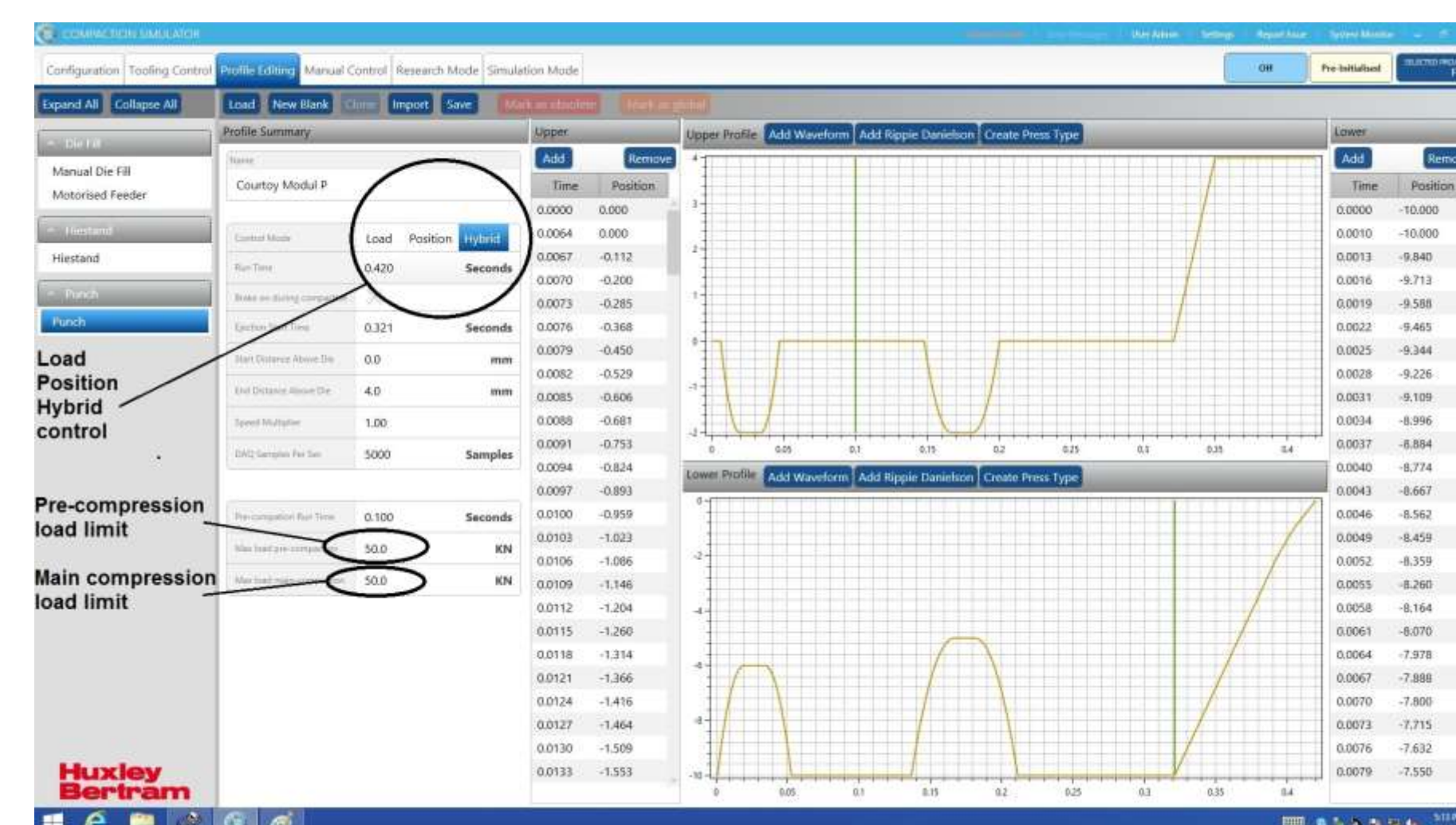
Setting up a hybrid controlled test in "Research Mode"
